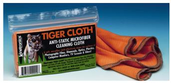
Anti-Static Tiger Cloth, The Kinetronics ASC-BP is an anti-static, microfiber cloth that has been specifically engineered for cleaning photographic films. The 10" x 18" (250mm x 450mm) orange cloth has stripes of effective conductive fibers knit every 1/8" or 4mm that dissipate or drain off static charges.
